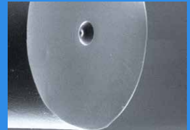
Figure 1. High purity synthetic silica fiber (OFS AllWave ZWP Fiber)
